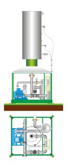
High efficiency, compact biogas suction and combustion unit mounted on a frame. Compact design and easy installation allow use in emergency situations, for temporary installations or to check the production capacity of the landfill.
