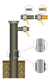
Used for definitive or temporary closure of biogas wells created by drilling or progressive growth during the landfill exploitation stages. Captures, regulates and transfers biogas from landfill.
