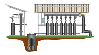
Connects wells or horizontal biogas capture lines, used to adjust biogas flow and check quality for each inlet line. It is fitted with fine flow adjustment valves and a condensate discharge system shared by all inlets located on the outlet from the main manifold.
