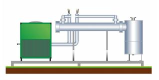
The system includes the equipment and instruments needed for initial treatment of biogas entering the motors to eliminate moisture content and, at the same time, reduce hydrogen sulphide content. It can be installed as standard equipment of the inlet system or assembled separately on a specifically designed chassis. The main components of the system are the biogaswater heat exchanger, the chiller and the condensate collection and discharge equipment.
